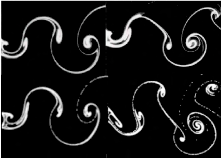
Figure 4.2: Experimental dye visualisation from Williamson & Govardhan (2004) (top) and results from particle tracking simulations (bottom) of the 2S mode (left) and the P + S mode (right). The comparison between the two is very close, and indicates that the P + S mode in particular is physical.
