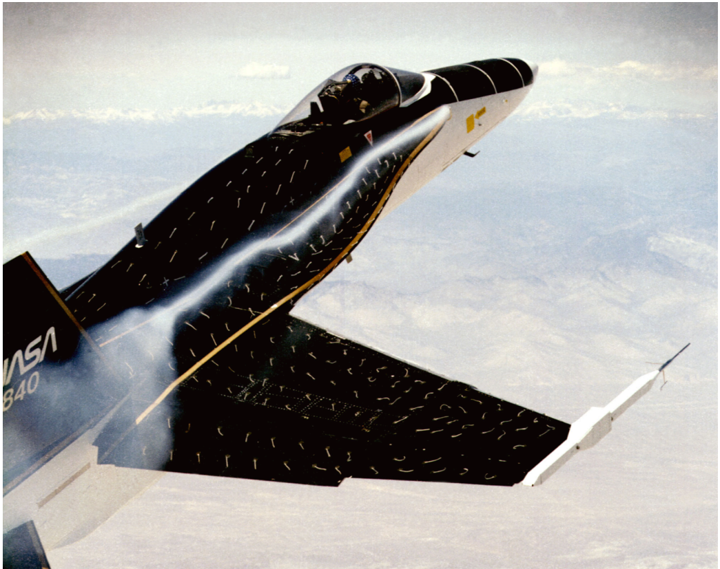
Figure 1.1 NASA F/A-18 Research vehicle at 20 degrees angle of attack showing a strake vortex using smoke. The picture also shows vortex breakdown towards the trailing edge.
