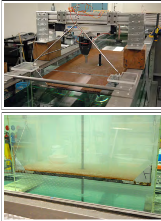
FIGURE 3.10: A photograph showing the honeycomb used to settle the flow for the quiescency experiments.
