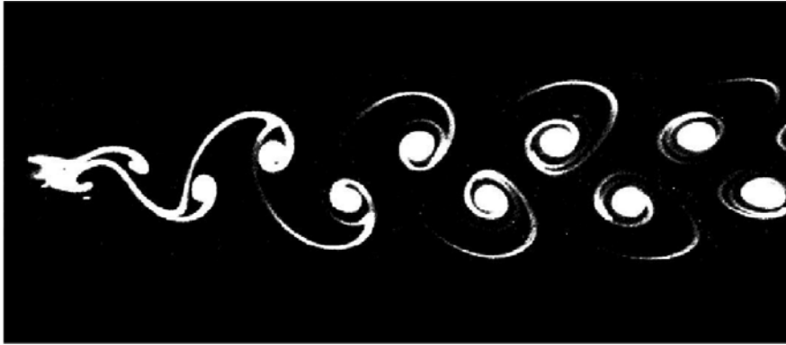
FIGURE 2.1: Kármán vortex street behind a circular cylinder at Re = 105 . The image shows streaklines produced by electrolytic precipitation in water. Photograph by Sadatoshi Taneda and is then reproduced from Van Dyke (1982)
