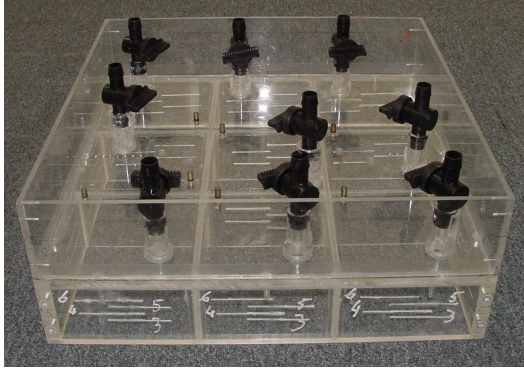
Figure 3: The nine compartment air-cushion box model, 9-C.
