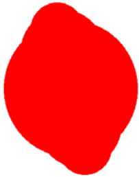
Figure 7: Typical shape of an ellipsoidal particle assumed in the current study. Combining multiple spheres of different diameter forms particle.
