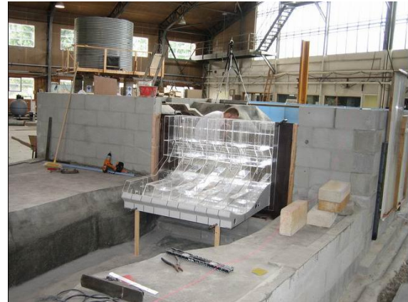
Figure 1: A photograph of the four bay radial gated spillway used in the physical model testing.
