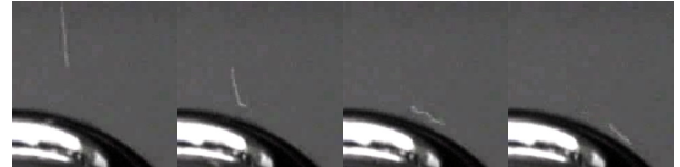
Figure 3: Sequence of images illustrating a spherical \sim 125 \mu\text{m} particle (soda–lime glass Ballotini ) rebounding from the surface of a \sim 2.0 \text{ mm} bubble. Particles were ejected from a pipette with a high velocity. The particle’s movement means only a bright spot shows up at its centre (the particle focuses light from behind). The interval between successive frames is 40 ms, and the exposure time is slightly shorter.
