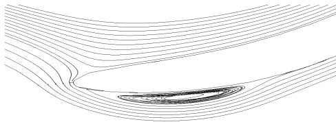
Figure 4: The streamlines near the leading edge, M_{2is} = 0.99
