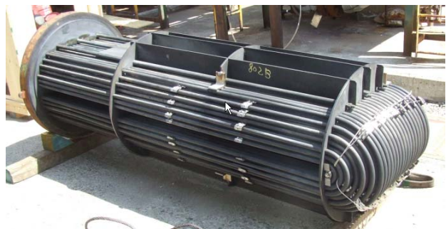
Figure 2: DTS Strips Applied as U-Bend Stiffener.
