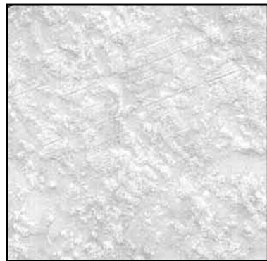
Figure 9: The defective tile image for Crack defect
