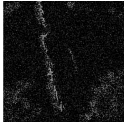
Figure 14: Variance for Daubechies Wavelet for Crack defect tile image
