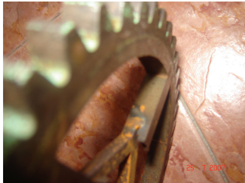
Figure 1: The welding section on the mild steel gear
