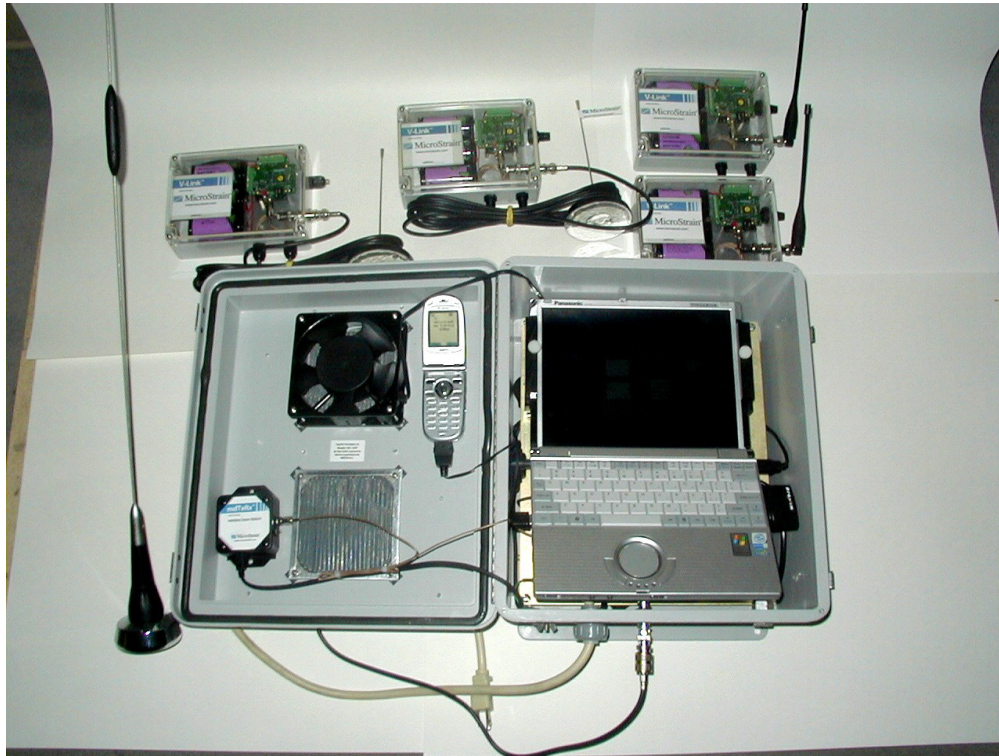
Figure 2. Wireless Sensing Nodes (4) in sealed NEMA 4X enclosures (top). Base Station with Panasonic Toughbook®, cell phone, 802.11b WiFi card, and narrowband RF Transceiver as packaged within sealed, thermally controlled enclosure (bottom).
