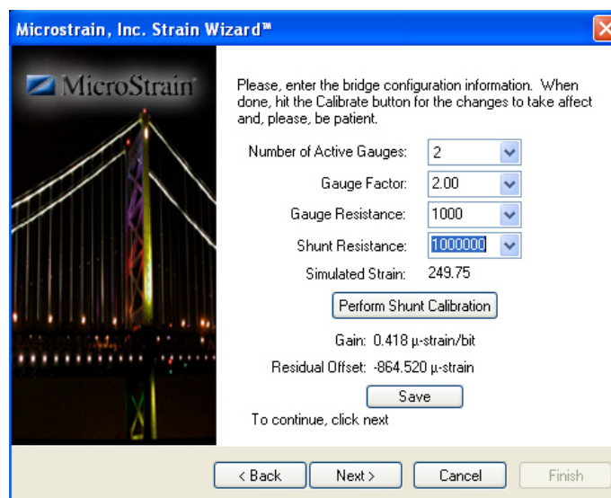
Figure 8. Software interface to provide the user with requisite gain and offset values after the remote balancing & shunt calibration steps have been performed.
