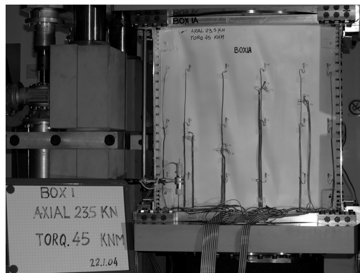
Figure 6 – The collapse picture of the box
