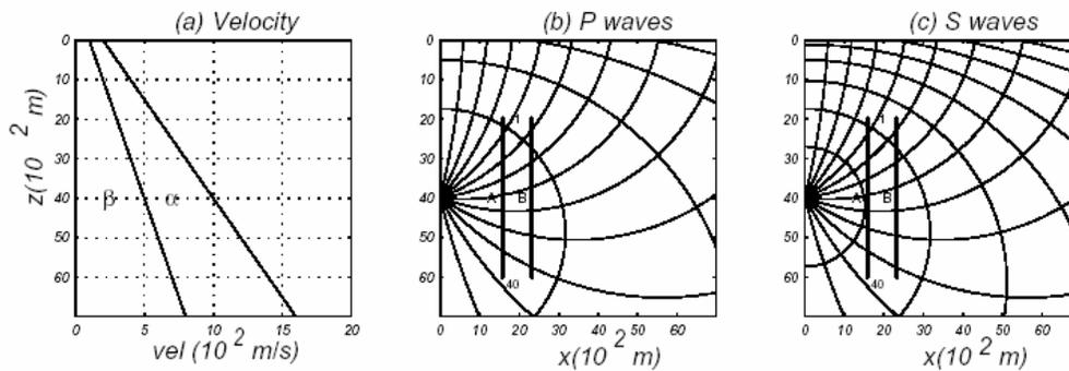
Figure 2.- Properties in a heterogeneous medium a) velocities  $\alpha(0)=200m/s$ ,  $\beta(0)=100m/s$ ,  $\rho(0)=1T/m^3$  and  $h=1000$  m, b) and c) rays and wavefronts every 3 s. Set of stations A and B in thick line.
