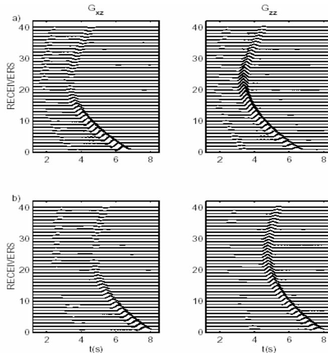
Figure 3.- a) and b) Displacements in a heterogeneous medium for a vertical force in the receptors sets A and B. Material properties and positions of both source and receivers are shown in Fig. 2. In continuous line the exact analytical solution and in dotted line the solution obtained with a fourth order FDM.
