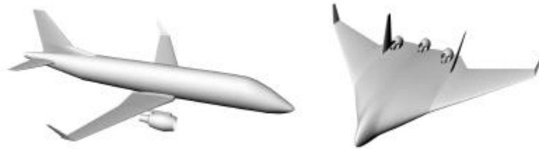
Figure 3 Commonality between different aircraft configurations captured with KBE based Parametric Modelling
