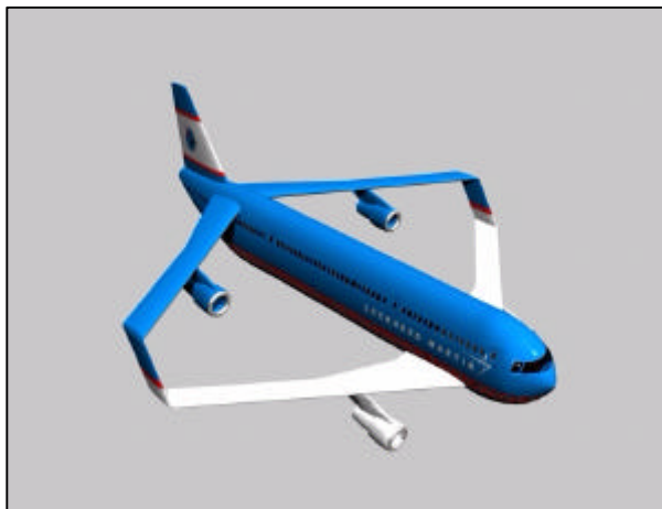
Figure 13 A box-wing aircraft configuration
