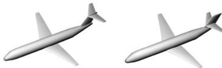
Figure 4 Variation within an aircraft type captured with KBE based Parametric Modelling
