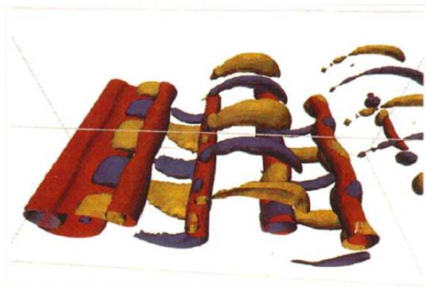
Figure 1.10: Iso-surface visualization of a Mode A instability from a direct numerical simulation; the yellow surface represents positive \omega_x ; the blue surface represents negative \omega_x ; the red surface represents \omega_z ; from Thompson et al. (1994)
