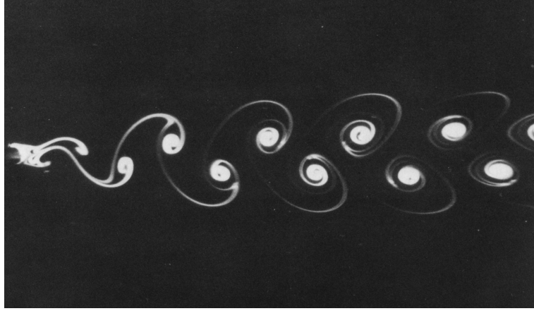
Figure 1.2: Karman vortex street in the wake of a circular cylinder at Re = 105 ; Van Dyke (1982)
