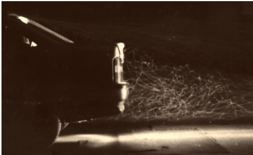
FIGURE 2.2: Turbulent flow inside the near wake of a car. Photo: Opel from Tropea et al. (2007) .
