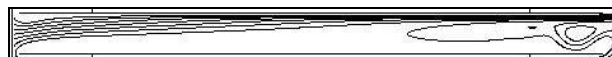
Figure 7: Streamline plot of the flow in the air gap with a height of 0.14m and an inclination angle of 25°.
