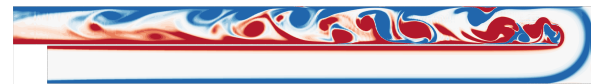
Figure 9. Unsteady flow at H = 400 , Re = 3000 without the presence of secondary recirculation bubble prior to Re_c .
