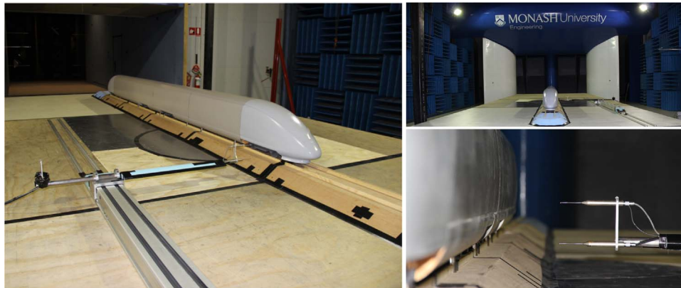
Fig. 6. The experimental configuration of the cobra probes mounted on streamlined and balanced arms, and moved with a computer controlled traverse. This setup was used to obtain streamwise measurements to develop slipstream profiles.
