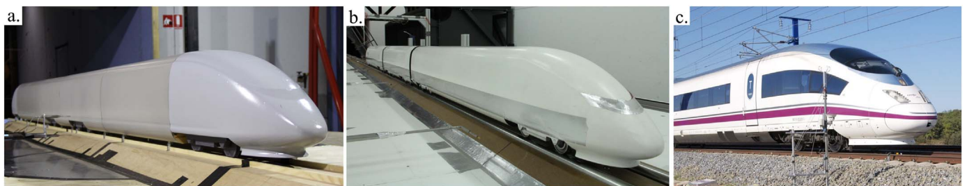
Fig. 2. The Inter-City-Express 3 high-speed train geometry investigated: (a) 1/10th-scale wind-tunnel model, (b) 1/25th-scale moving-model, (c) full-scale operational train (Photo provided courtesy of Bombardier Transportation).
