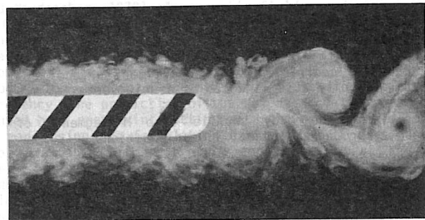
Fig 3: Flow visualisation of observed wake at acoustic phase angle comparable to Fig 2b.
