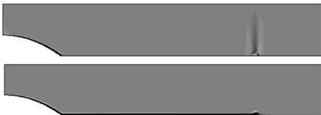
Fig. 4 Contours of vertical (top) and radial (bottom) velocity depicting dynamic locality and boundary layers respectively for Re = 11266 . Greyscale contours are used where light and dark shadings denote positive and negative values respectively.
