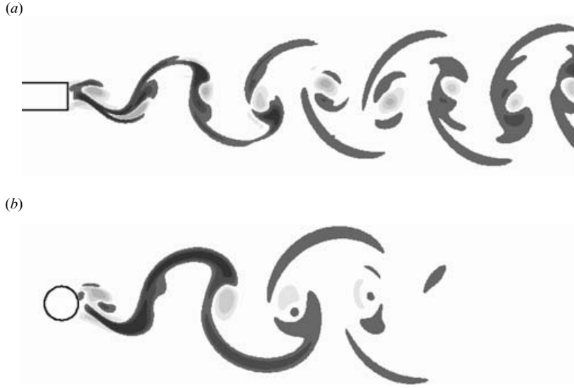
FIGURE 9. Comparison of the wake streamwise vorticity field of the Floquet mode for the elliptical leading-edge cylinder ( AR = 7.5 , Re = 450 , \lambda = 2.2H ) and the circular cylinder ( Re = 259 , \lambda = 0.8D ) showing the same spatial symmetries.
