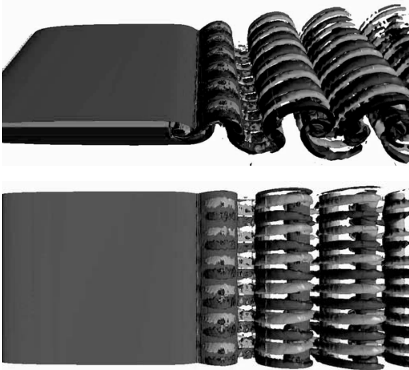
FIGURE 20. Streamwise vorticity contours from three-dimensional DNS calculation for AR=12.5 and Re=600 showing Mode B instability. ■ and ■ iso-surfaces represent \omega_x , ■ iso-surfaces represent \omega_z the cylinder is shown as ■.
