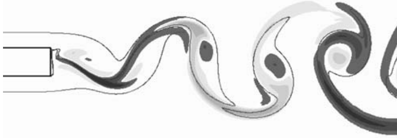
FIGURE 11. Streamwise vorticity field of the Mode S' instability ( AR = 7.5 , Re = 500 , \lambda = 1.0H ). The positions of the Kármán vortices are highlighted by the contours of spanwise vorticity of the base flow at \omega = \pm 0.2 .
