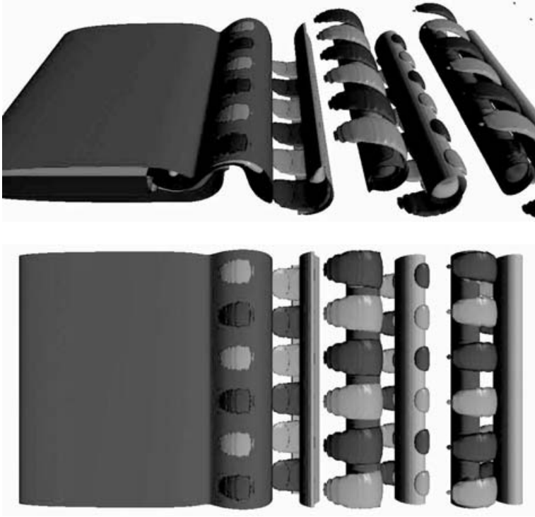
FIGURE 17. Isosurfaces of the streamwise vorticity field for the Floquet Mode A. Isosurfaces of spanwise vorticity ( \omega_z = \pm 0.2 ) are also shown to indicate the positions of the Kármán vortices. ( Re = 400 , AR = 7.5 ).
